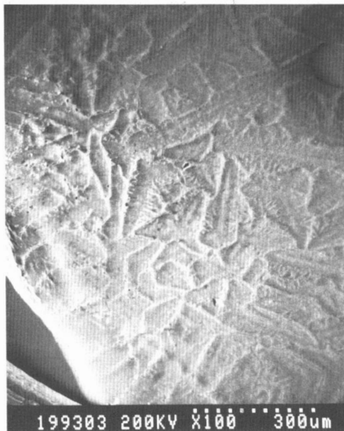
Figure 2. SEM image of the NdCo 8 B 3 Si film ( \times 100 ).
